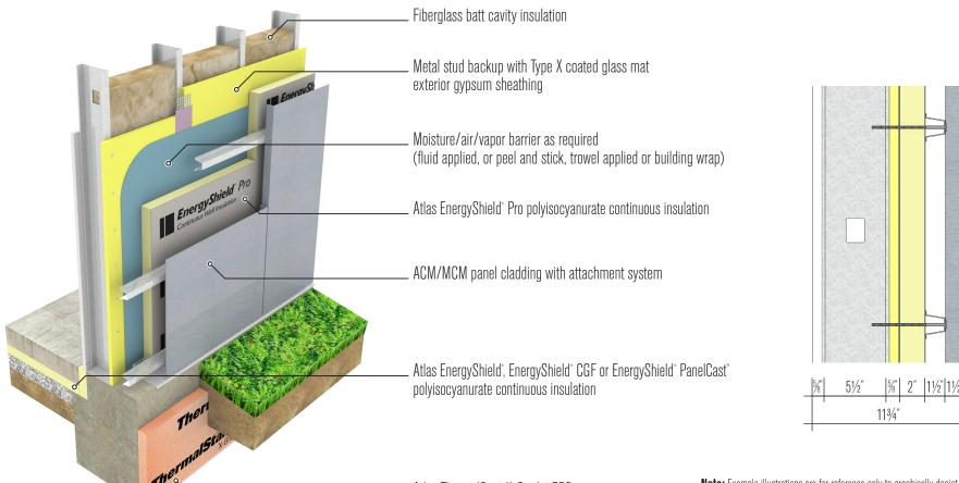
Atlas ThermalStar\* X-Grade\* FPS rigid continuous insulation at foundation **Note:** Example illustrations are for reference only to graphically depict location of Atlas manufactured materials in relationship to other materials in a wall assembly. The images are not intended for construction documentation. A registered professional must review for accuracy and approve fitness for intended use. These images are the property of Atlas Roofing Corporation.
